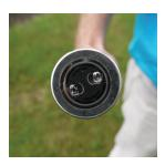
A VisoTurb sensor with UltraClean technology remains clean after a 30-day deployment.
